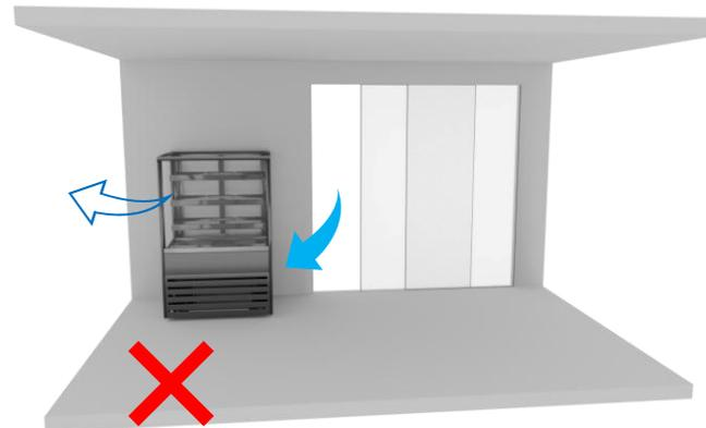
As standard, units are self evaporating to a receptacle in the condenser unit. In a new site where external drainage is accessible, it is recommended by-passing the evaporation dish. A plastic hose can be attached to the end of the condensate drain and re-directed as shown. This reduces power consumption and will result in less maintenance being required over time.
