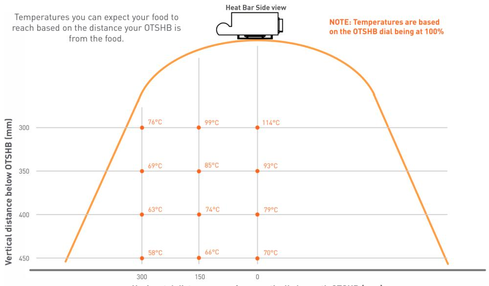
Horizontal distance away from vertically beneath OTSHB (mm)
