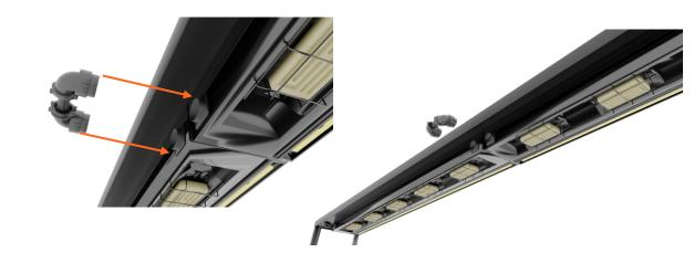
Once the heat bars have been installed into the pass-through end-to-end, a connecting cable can be plugged into the end sockets of each heat bar. Doing this allows up to 3 heat bars to run in series off one larger electrical box, one controller and one power cable.
