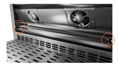
Reattach the bracket screws at either end of the element
