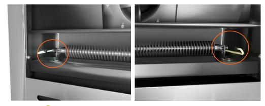
Unplug the wires from the element terminals at either end
