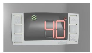
When on, this green symbol means the compressor is on
