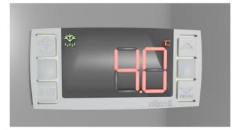
When flashing, this green icon means the cabinet is defrosting
