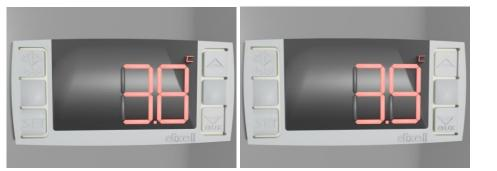
Press the up or down arrows to change the temperature. Press the SET button to lock in your chosen temperature
