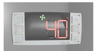
When on, this green symbol means the airflow fans are on
