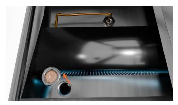
Lift the drain net out of the drain
