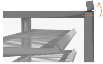
Pull the front top trim forward and rotate upwards
