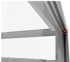
Replace the top screw of the rear edge panel (RF only)
