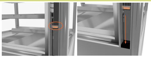
Unclip the heated wire from the connection in the rear pillar and feed the wire back through the hole at the base of the pillar (RF only)
