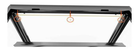
Remove the screws that attach the top bracket to the cabinet and remove the bracket from the cabinet
