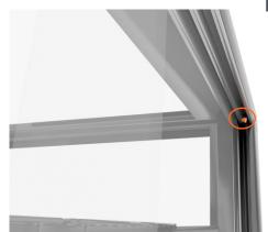
Remove the top screw located on the edge of the panel by the top door track (RF only)
