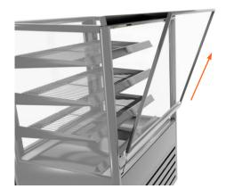
With the front glass tilted forward as far as it can, lift the front glass with glass bracket upwards with the heated wire pulling through the cabinet frame
