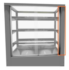
The rear right panel needs to be removed to allow access to the heated wire connection (RF only)
