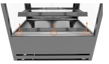
Remove the screws that attach the base bracket to the cabinet and remove the base bracket
