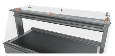
Place washers on top of the top glass at the rear, in line with the holes in the glass
