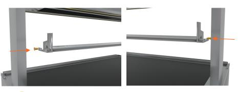
Attach the front side glass holders to both ends of the front hinge bracket
