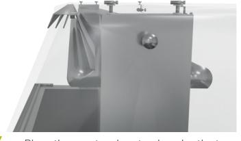
Place the rear top door track under the top glass, lining the attachment holes up with the holes in the top glass
