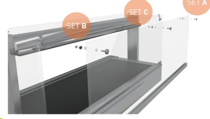
Prepare the front glass to be installed by attaching the front glass screw assemblies (see next page)
