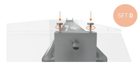
Place rubber washers on top of the top glass and secure the glass to the pillars with M5 22mm lugs
