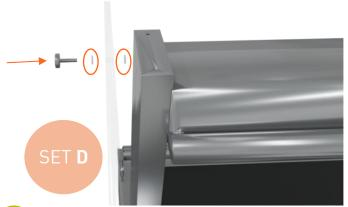
Screw the top of the left side glass into the gantry post using a M5 22mm lug with a rubber washer on both sides of the glass
