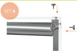
Attach the front right bracket to the side and top glass using M5 16mm lugs. Ensure rubber washers are on both sides of the side and top glass
