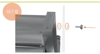
Screw the top of the right side glass into the gantry post using a M5 22mm lug with a rubber washer on both sides of the glass
