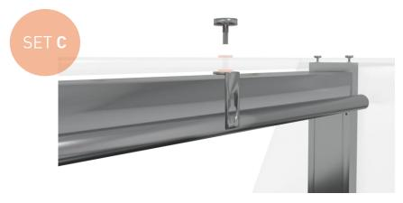
(LS5/6 ONLY) Attach the front middle bracket to the top glass using a M5 16mm lugs. Ensure rubber washers are on both sides of the top glass
