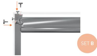
Attach the front left bracket to the side and top glass using M5 16mm lugs. Ensure rubber washers are on both sides of the side and top glass
