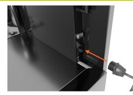
Plug the power cable into the side of the screen
