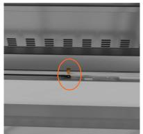
Pull the left retractable wire out of its housing and reinstall it on top of left door using screw previously removed
