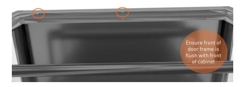
Mark, drill and tap the outer row of holes in the top of the frame (shown in green). Brush away metal shavings and insert screws
