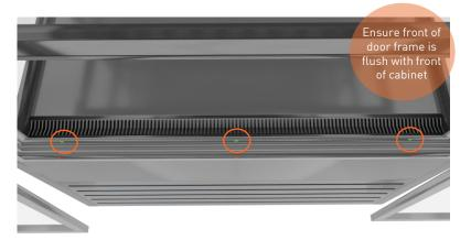
Mark, drill and tap the inner row of holes in the base of the frame (shown in green). Brush away metal shavings and insert screws
