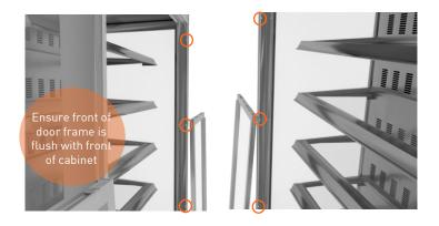
Mark, drill and tap the outer column of holes in the sides of the frame (shown in green). Brush away metal shavings and insert screws
