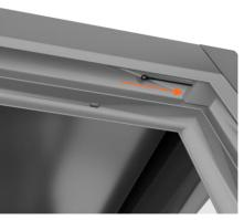
Unscrew the retractable cable from the top of the right door. Let the cable retract back into its housing. Place door to the side
