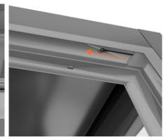
Pull the right retractable wire out of its housing and reinstall it on top of right door using screw previously removed
