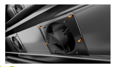
Screw the fan plate back onto the cabinet
