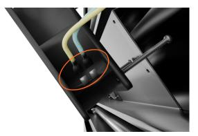
Unplug the wires from the terminals on the fan
