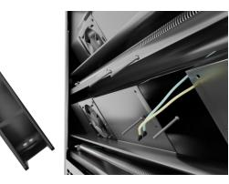
Remove the old fan and have the new fan ready to be installed
