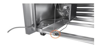
Ensure the cable runs through the grommet in the cabinet frame
