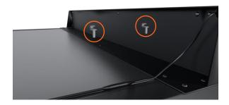
Use the supplied cable clips to secure the lightbox extension cable to the cabinet
