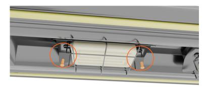
Reattach the wire guard to the heater housing using the same two screws
