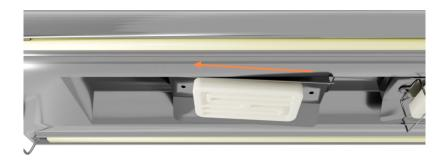
Slide the housing to the side to lock it in position in the gantry
