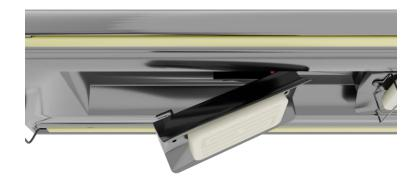
Place the heater housing back into the gantry, making sure not to crush any of the wires
