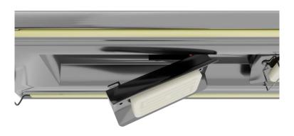
Move the housing to one side before pulling it down to release it from the gantry
