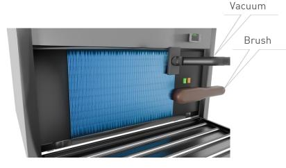
Using a brush or vacuum with a brush attachment, sweep up and down the condenser face only, not horizontally
