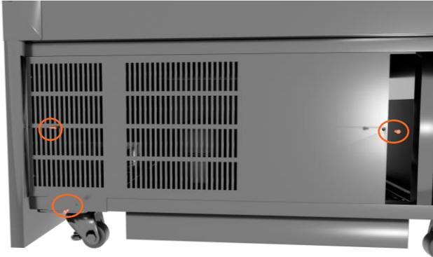
**3** ■ Remove the screws that hold the rear grill on to the rear of the cabinet and move the grill out of the way
