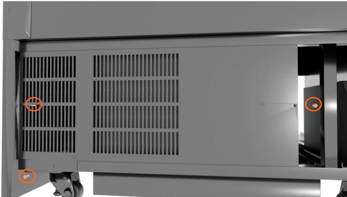
**13.** Place the rear grill back into position and reinstall the screws
