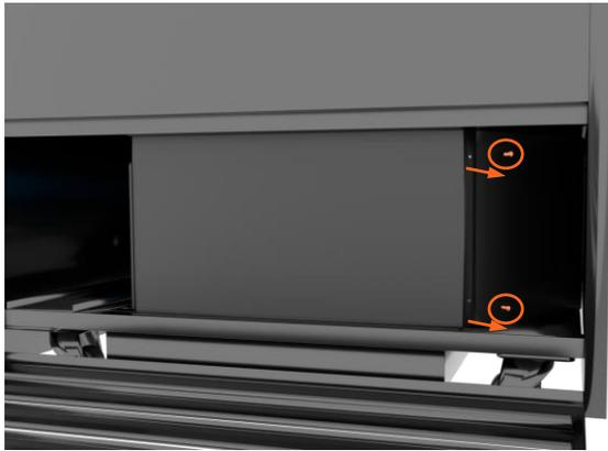
**5** ■ Remove the screws attaching both baffle pieces together. The front baffle piece can then be removed from the front of the cabinet
