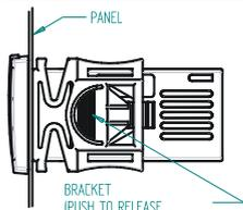
Instrument XR70CX shall be mounted on vertical panel, in a 29x71 mm hole, and fixed using the special bracket supplied. The temperature range allowed for correct operation is 0 to 60°C. Avoid places subject to strong vibrations, corrosive gases, excessive dirt or humidity. The same recommendations apply to probes. Let air circulate by the cooling holes.
