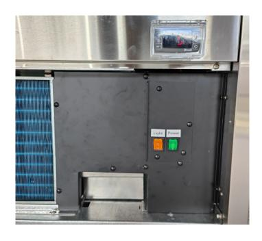
7. Install the electronic box back to the front panel Install the back metal panel Turn on the power Install the front grill back
