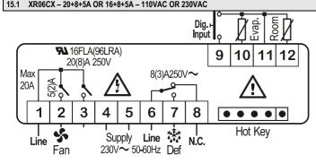
NOTE: The compressor relay is 20(8)A or 16(6)A depending on the model. NOTE: Connect the 120Vac power supply to 4-5
