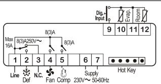
NOTE: Connect the 120Vac power supply to 6-7
