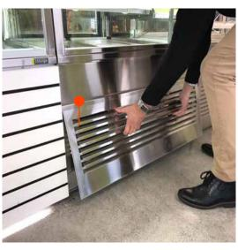
Turn off the power and remove the grill in the front
