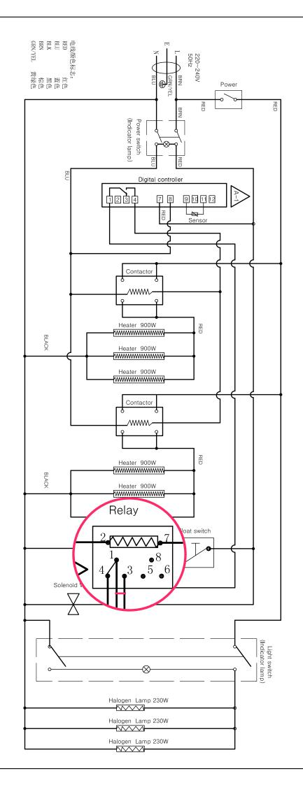
To run unit with out water Remove no 1 and 3 Wires from relay And join them together with Conecter block
