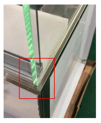
Mark down four corner position Using knife cut the double sided tape between the glass and steel
