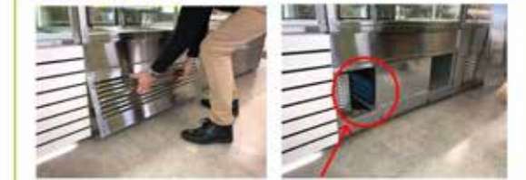
Remove Grill to access condenser
