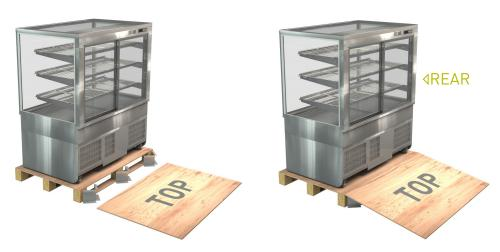
Place three or four of the corner brackets on a level floor in front of the bottom pallet with the **rear of the cabinet facing the ramp.**Place the plywood top cover on the floor and corner brackets to form a ramp.
