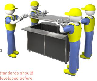
After unit has been placed in the required position remove the lifting bracket bolts and retain for fixing the gantry posts.
