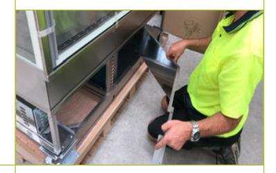
3. Remove drainage pipe
